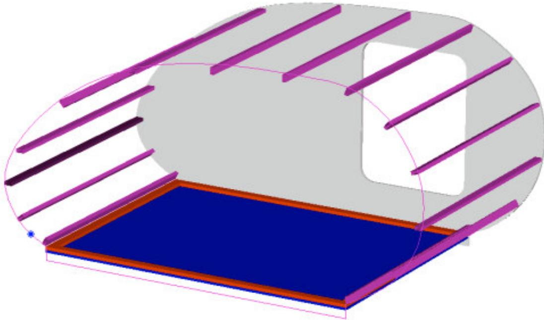
The placement of the stringers is not crucial. Space the stringers evenly throughout the camper. However, it is crucial that the stringers are located at the same place on both sides. The stringers should be mounted so they are flush with the edges of the camper.
