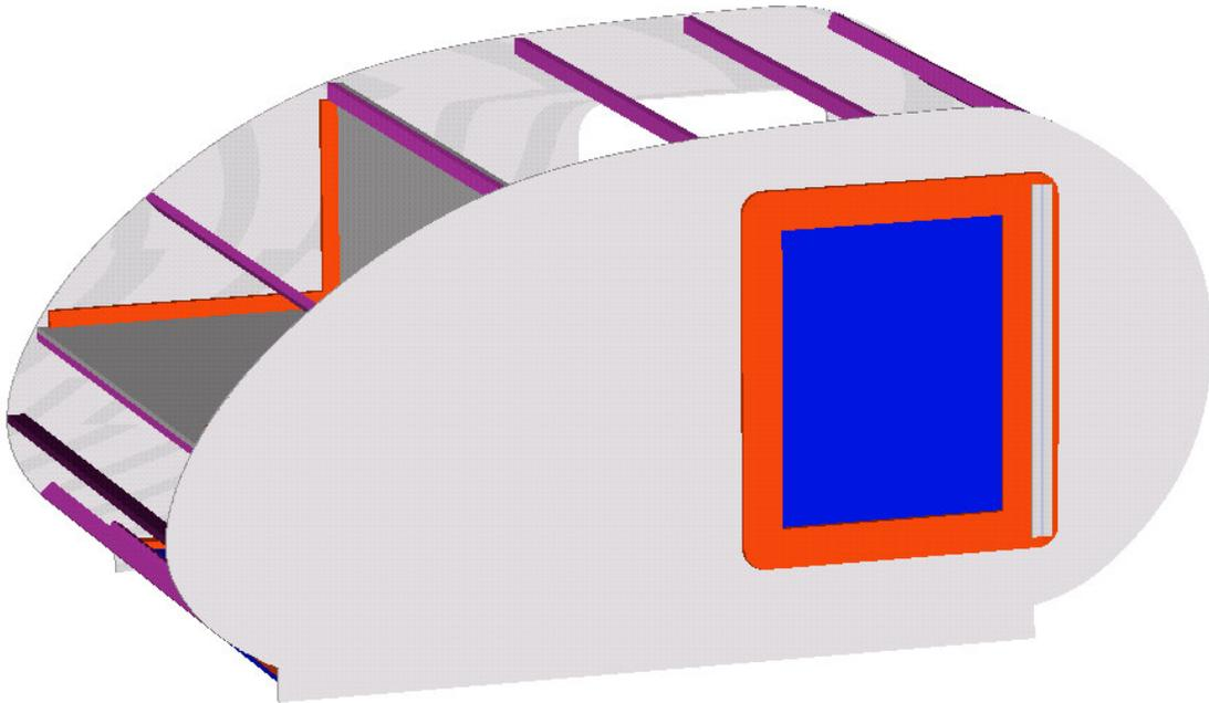
The 3/8" plywood doors should sit flush with the camper sides when the door is closed. The 3/4" door frame should sit tightly against the camper sides. The doors should always be hinged at the front of the camper.
