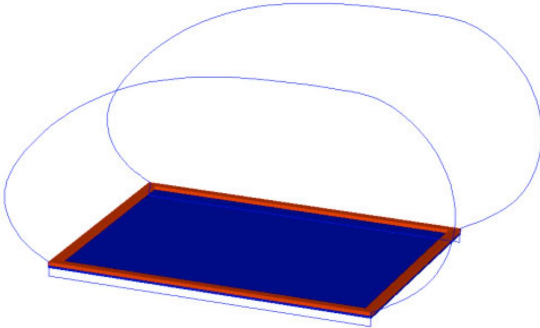
Toe rails (shown in red) are then cut from 1 x 2 stock and screwed to the floor (shown in blue) using 1-1/4" #8 wood screws. I placed a screw approximately every 6 inches. You will need to cut the toe rails:
