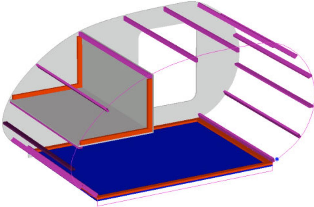
The cupboard stringers (shown in red above) will vary in length according to your setup. The cupboard stringers are constructed from 1" x 2" leftovers from the main stringers (shown in purple) of the camper. The cupboards (shown in dark gray) are attached to the stringers using 1-1/4" wood screws.
