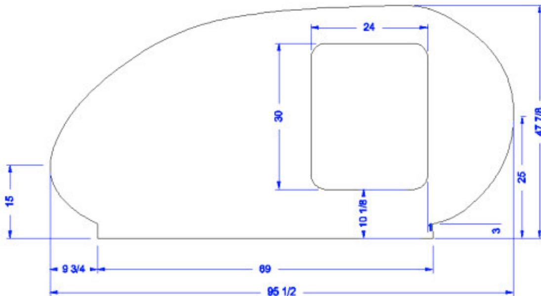
The doors measure 1" back from the front straight part of the camper which covers the trailer, and 10 1/8" from the bottom of the camper. If you decide to use a flush fitting door, then you will have no clearance problems with the fenders. If you use the overlapping doors, then they'll need to be modified to allow for the fenders. (This is assuming your trailer axle is in the same location as mine.)
