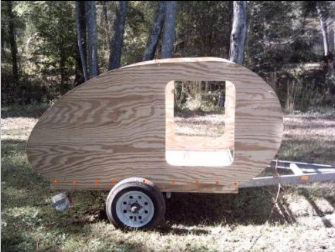
It's easier to scribe a line across the bottom location where the side will mount to the bottom. The straight line from the back of the camper to the front should be mounted so that the top of the floor (not the toe rails) is flush with the scribed line. Start from the back and pre-drill the holes. You will need to use a countersink/drill for this. Use the 2" coarse drywall screws to attach the sides to the toe rails.
