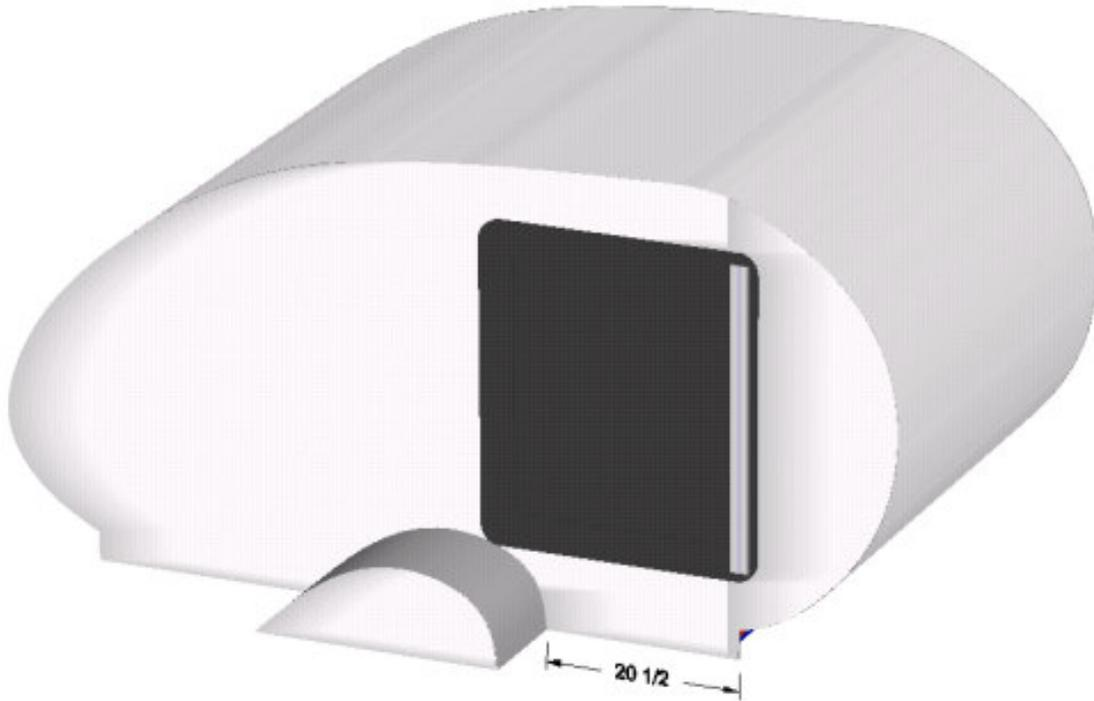
The fender is mounted 20-1/2" from the front trailer cover of the camper. This measurement will depend of the trailer used.
