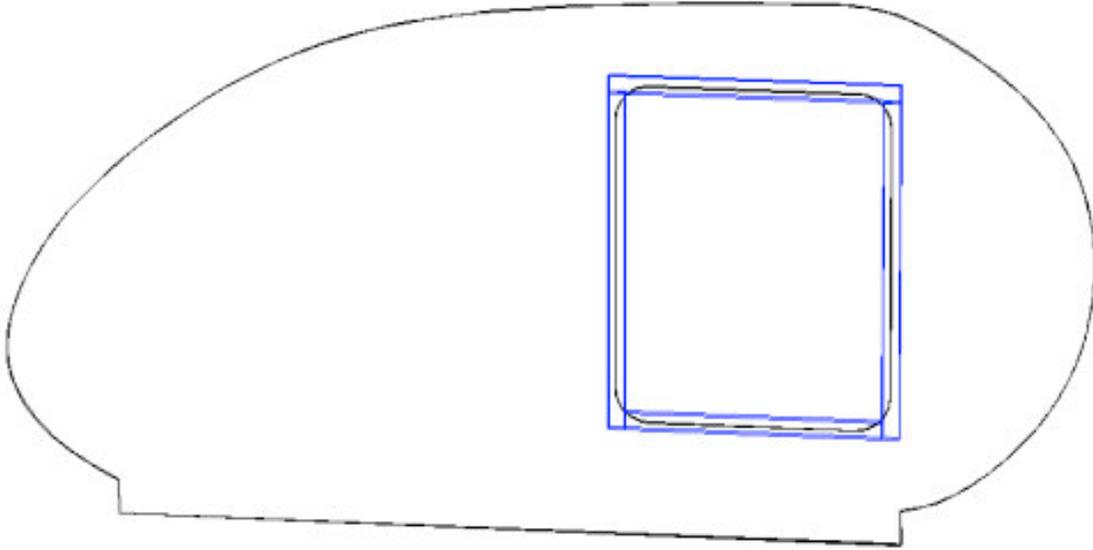
The next step in the door construction is to add the door jambs to the sides. The door jambs are constructed from 1" x 2" and are centered in the doorway so there is 3/4" overhang for the door to close on to. Countersink the holes on the camper sides, and screw the door jambs to the sides using 1-1/4" wood screws.
