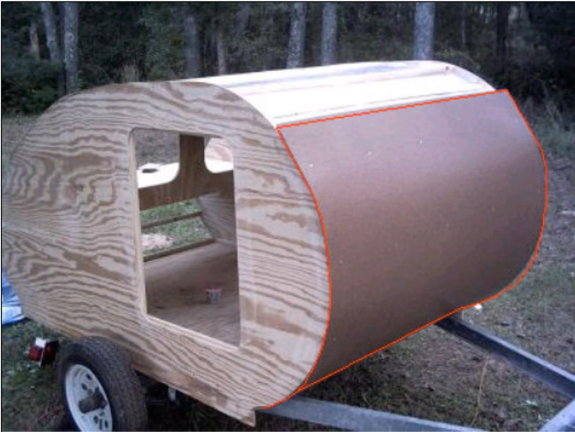
To join each section of hardboard to the previous, cut a 1" x 4" x 52" board and use 3/4" wood screws to mount it. You will need (3) 1" x 4" x 52" boards to join the 4 sections of hardboard. Use a countersink to keep the screw heads flush with the hardboard. Be careful not to countersink too deeply as the screws can pull through the hardboard.
